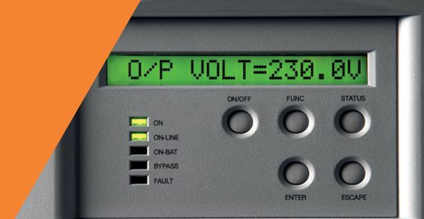
UPS systems of the type Wärtsilä JOVYTEC L are available with performance ranges of 6 kVA, 8 kVA or 10 kVA. Due to their online double converter technology these UPS systems meet the requirements of the highest protection class VFI-SS-111. During start-up a diagnostic system is activated verifying the status of the UPS system and the battery. The power related fan control system protects the system against overheating and ensures a long battery life.
